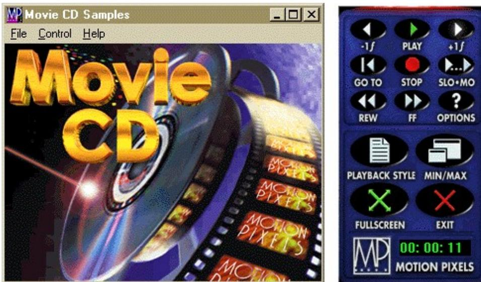
The Motion Pixels Movie CD Player automatically loads this configuration on the Windows desktop. The following is a description of the virtual remote control and its related functions. Please note that some Remote Control functions, such as rewind, fast-forward, and slow-motion, only work with the windowed video.
