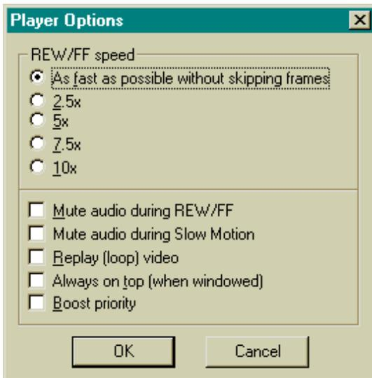
The "Rewind/Fast Forward Speed" can be adjusted to play as fast as possible without skipping frames. The other speed options are ratios of normal playback speed.
